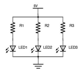
Identify the components that are in in the drawing above, and those that are in parallel: \*
